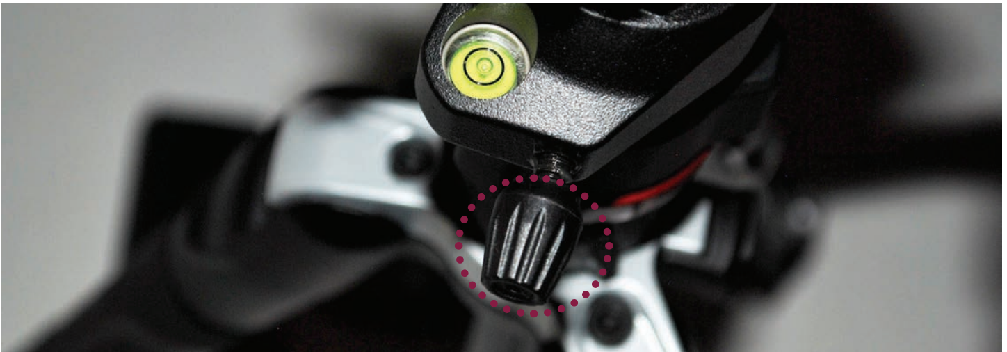
This is the pan lock knob , and it secures the side-to-side movement of the tripod head .
