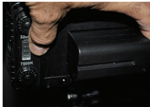
Lithium-ion battery inserted into backside of LED light
